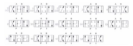
Most of these patterns can be implemented by selecting initial orifice openings in the four-orifice valve configuration shown in the previous section, in the figure named Modeling a 4-Way Directional Valve on page 2-34 (for example, patterns 0, 1, and 3). However, some patterns require a model with six or more variable orifices. For instance, pattern 4 can be implemented with the following configuration, which requires six variable orifice blocks.
