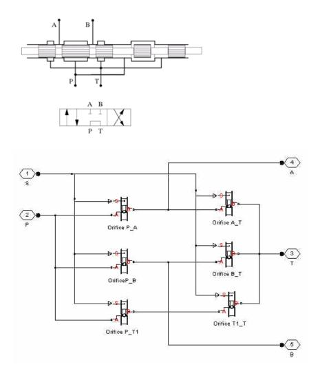
The Orifice with Variable Area Round Holes blocks have been used as a variable orifice in this model. Port T1 corresponds to an intermediate point between ports P and T.
