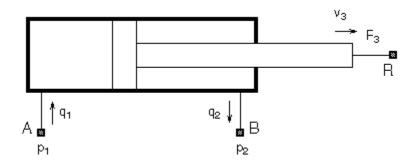
The element is represented with three energy flows: two flows of hydraulic energy through the inlet and outlet of the cylinder and a flow of mechanical energy associated with the rod motion. It therefore has the following three connector ports:
