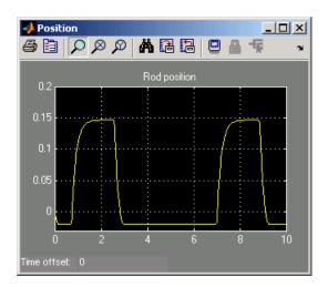
As you see, in the beginning the valve is closed. Then, as the input signal reaches 50% of the actuator's nominal signal, the valve gradually opens to its maximum value and moves the cylinder rod in the positive direction. When the input signal goes below 50% of the nominal signal, the actuator closes the valve. The spring returns the cylinder rod to its initial position.
