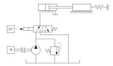
The power unit consists of a motor, a positive-displacement pump, and a pressure relief valve. Depending on its characteristics, such a power unit can be modeled in a variety of ways, as described in "Modeling Power Units" on
