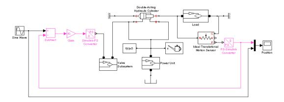
A better way to avoid an algebraic loop is to use physical signals for the controller, as shown in the modified model below.
